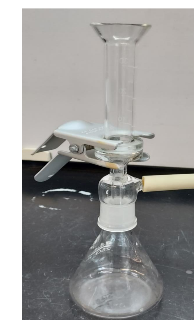
Figure 4: Vacuum filtration set up with a removable 5-micron stainless steel filter
