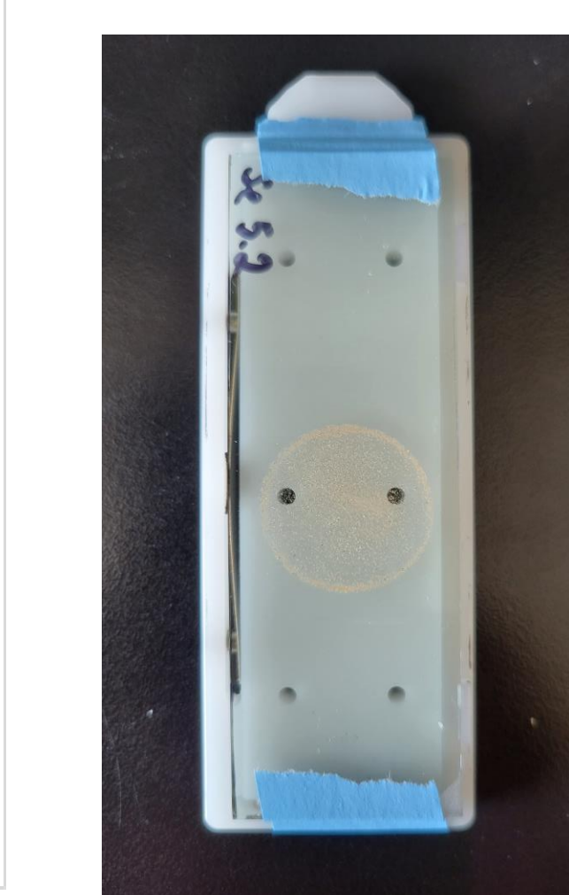
Figure 6: Kevley slide with sewer sample prepared.
