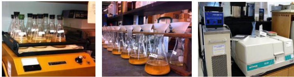
Figure 2. Extracting nitrate from resins and nitrate determination in the lab
