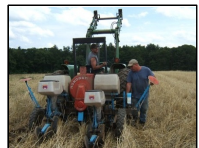
Farmers at ME-WA planting squash with a deep zone tillage (DZT) implement borrowed from UMass.
