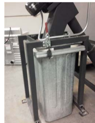
Ash is injected into bin and emptied monthly
