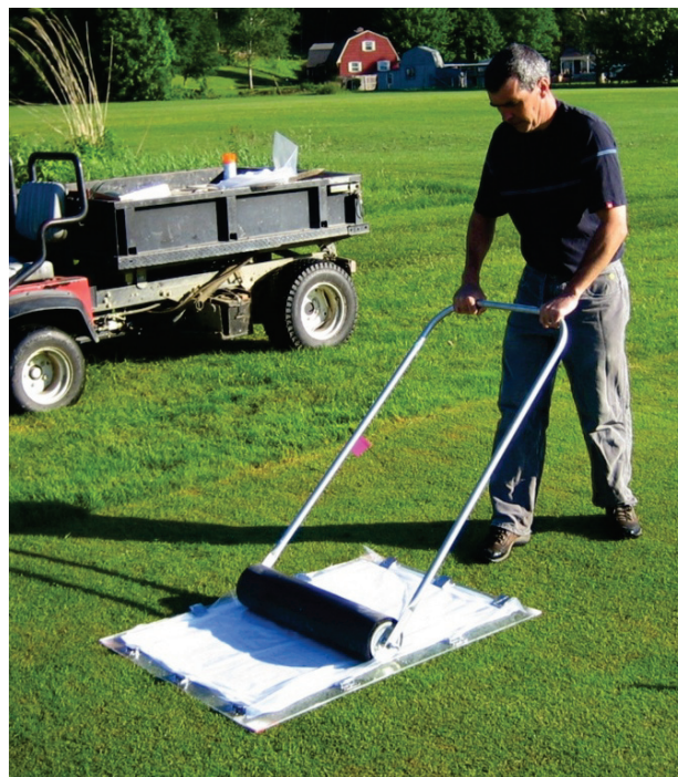
Figure 5. Dislodgeable foliar residues (DFR) were collected with a California roller (CA roller). A 6 ft 2 piece of cloth was placed over a frame and the 32-lb CA roller was slowly rolled across the cloth 10 times. Pesticide residues were considered dislodgeable if they were transferred to the cloth.
