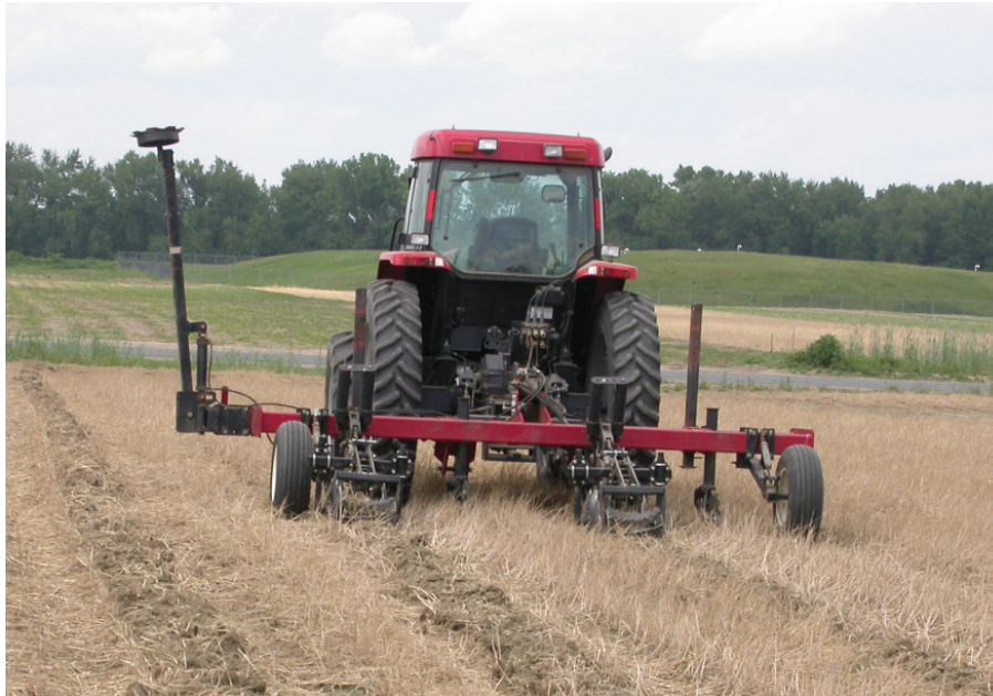
FIGURE 21 Deep zone tillage into a winter rye crop which was killed in early spring. Courtesy of Andy Cavanagh
