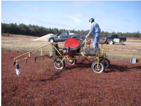
Fig. 3. G ephardt drop spreader delivering granular herbicide to the cranberry farm surface. Note white droplet of foam at left, which helps to guide the driver. Photo courtesy R. Gilmore.
