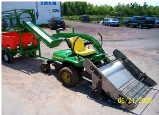
Fig. 3. Example of a tractor-driven dry harvester used to pick cranberry fruit. Photo courtesy D. Bragg, www.dbe.ca .
