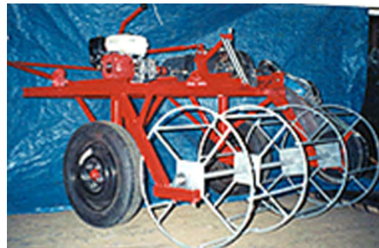
Fig. 4. Wet harvester (water reel) used to harvest cranberries in shallow floods. Photo courtesy F. Caruso.
