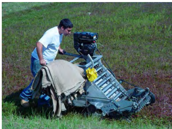
Fig. 5. Dry harvesting with a Furford picking machine that prunes vines as well as picks fruit. Photo courtesy B. Wick.
