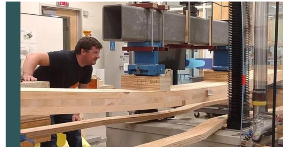
Picture 24. Research into Cross Laminated Timber Products Made from Eastern White Pine and Eastern Hemlock. Photo credit: Dr. Peggi Clouston, UMass-Amherst
