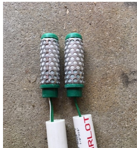
Soil Moisture sensors are used to track soil moisture levels for better crop production. Photo: J. DeLisle
