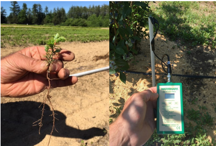
Sensor depth can be adjusted depending on the rooting depth of the crop. Photo J. DeLisle
