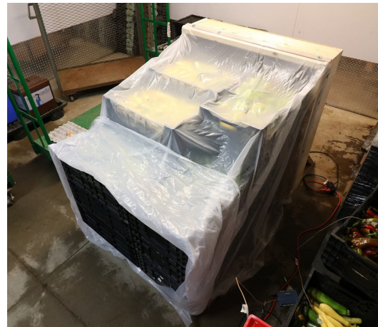
A floor pallet forced air cooler. Photos: UVM Extension
