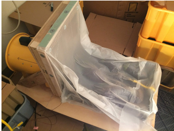
A countertop forced air cooler for 1-3 cartons of product. Photo: UVM Extension
