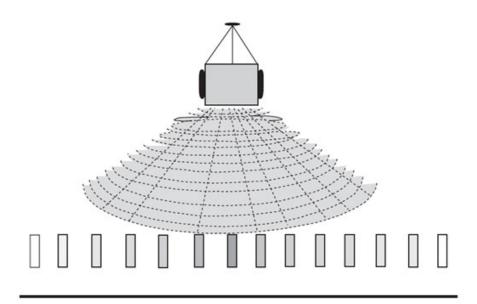
**FIGURE 4.** Actual fertilizer material distribution pattern using a rotary spreader and a 19-19-19 fertilizer.
