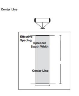
**FIGURE 3.** Check rotary spreader swath width and material distribution patterns using equally spaced containers (ice trays, empty egg cartons). Color of the collection trays is directly proportional to the amount of material collected (darker = most material).
