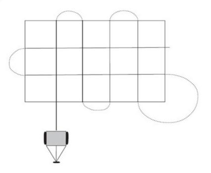
To conduct the test, fill the spreader at least half full, set it at the suggested spreader setting, and make three passes in the **same direction** over the boxes using normal walking speed. Weigh the material or put the material from each box into a test tube, vial, or small narrow bottle. When the bottles are placed side by side in order, a plot of the distribution pattern is
